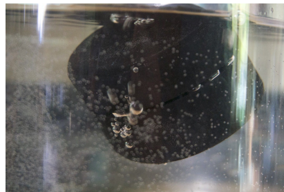
Waterproofing test in vacuum pump low pressure environment
